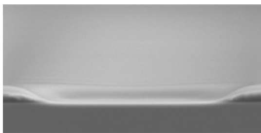
(a) Via Opening, Softbake = 120°C Sidewall Angle = 32° CD = 45 \mu\text{m}
